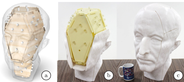
Figure 5.9: Avoiding support material: CofiFab [Song et al., 2016] splits the model into parts that do not require support, but the user has to assemble them at the end.
