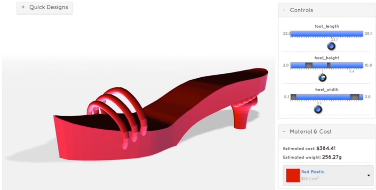
Figure 3.14: Parametrized Fab Forms [Shugrina et al., 2015] allow exploring only the physically valid options.
