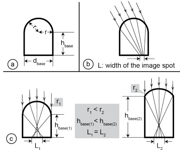
**Figure 7: (a) Basic lens parameters: lens diameter  $d_{base}$ , radius  $r$  and substrate height  $h_{base}$  (b) image spot  $L$ : the area underneath the lens that can be seen from one specific viewing angle, (c) to achieve the same image spot size, a smaller radius (i.e., more curvy lens), requires a smaller height.**
