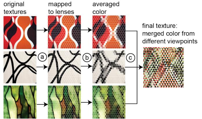
**Figure 11: Mapping color pixels onto lenses for each 3D texture: (a) Find which pixels are underneath which lens for each texture. (b) For each texture, average the color underneath each lens. (c) Divide the space underneath each lens using ray-tracing and assign the averaged color of the corresponding texture for each lens.**
