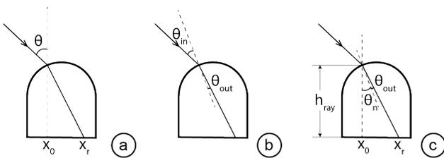
Figure 17: (a) A ray is defined with its direction  $\theta$  and its intersection coordinate  $x_0$  with the lens surface; the goal is to find the coordinate  $x_r$  where the refracted ray intersects with the lens's backplane. (b) Compute the incident  $\theta_{in}$  and refracted angle  $\theta_{out}$ . (c) Find  $x_r$  with  $\theta_{out}$ .
