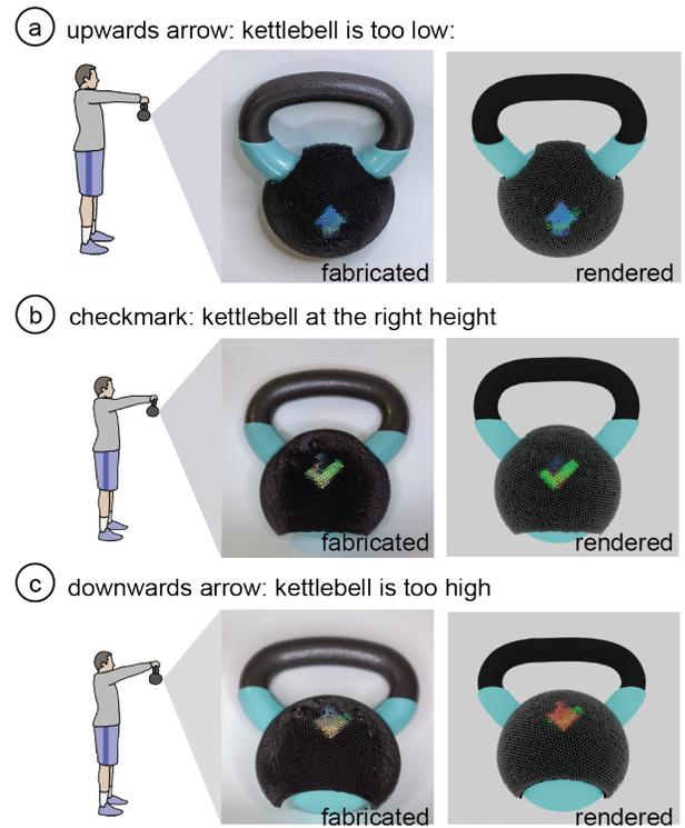
**Figure 12: Pose Guidance: this kettlebell guides the user to a correct front raise pose by displaying arrows when the kettlebell is too high or too low and a check mark when the kettlebell is at the right height.**
