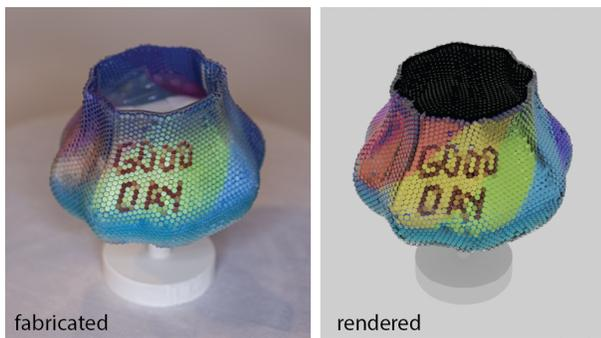
Figure 13: This lampshade displays different greeting messages when the users looks at it from different heights (laying down in bed vs. sitting up in bed).
