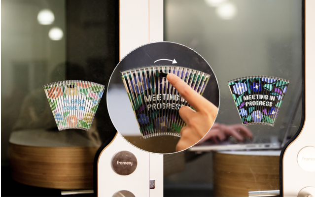
Figure 13: A fan-shaped door sign with an embedded ShiftLens structure. Flipping the switch shifts the lens layer to display either “Please Come In” (left) or “Meeting in Progress” (right), providing a passive, electronics-free status indicator.
