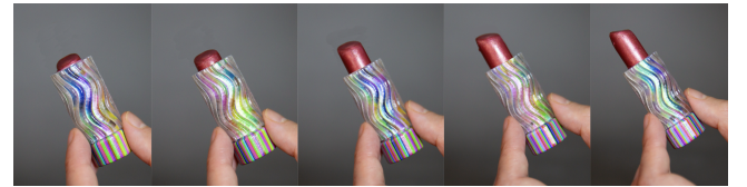
Figure 15: A lipstick tube with a ShiftLens structure driven by a roller mechanism. Rotating the barrel to extend or retract the product shifts the lens layer along the sine-wave surface, cycling the outer casing through a continuous color gradient.
