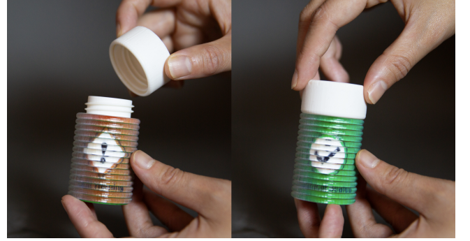
Figure 11: A chemical bottle with an embedded ShiftLens structure. The cap’s outer rim pushes the lens layer: a loose cap reveals a hazard warning symbol (left), while a fully tightened cap shifts the lens to display a checkmark (right).
